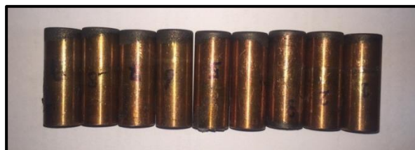
Fig.3 : shown copper electrode after cutting process
