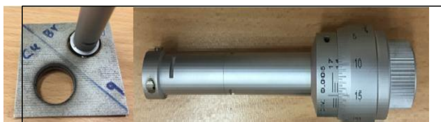
Fig.7 : Micrometer used for hole.
