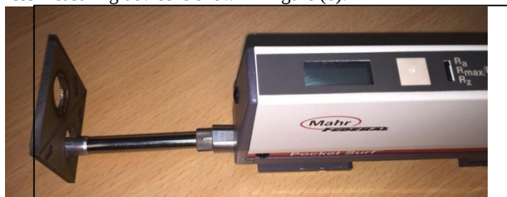
Fig.6 : Automatic digital POCKET SURF EMD-1500.
