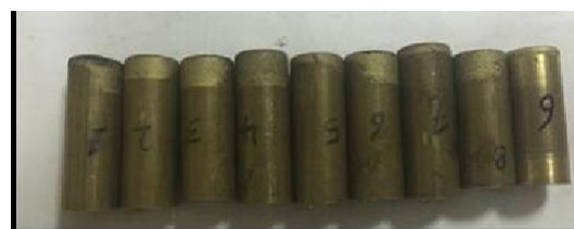
Fig.4 : shown brass electrode after cutting process
