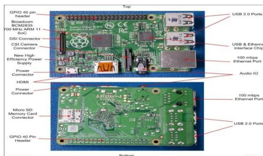
Fig..2 The Raspberry Pi B+ Board
